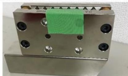
② Insert it from the top of the SSD destruction adapter with the longitudinal direction vertical:
