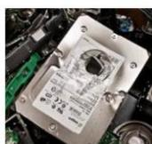
**Destruction:** Data around the center of the platters completely destroyed.
