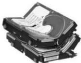
**Destruction:** Data along bend line completely destroyed.
