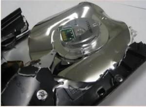
**Destruction:** Complete bending, and distortion of entire platter area leading to total data loss. This means that EVERYTHING and EVERY COMPONENT on a hard drive is targeted and demolished.
