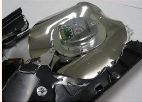
**Destruction:** Complete bending, and distortion of entire platter area leading to total data loss. This means that EVERYTHING and EVERY COMPONENT on a hard drive is targeted and demolished.
